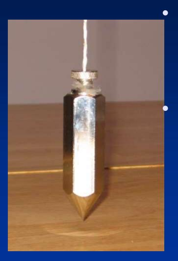
"A weight with a pointed tip on the bottom that is suspended from a string and used as a vertical reference line."
